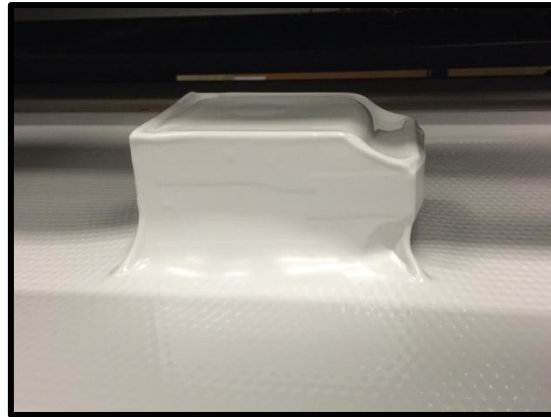
Figure 34 Vacuum forming the tote vessel
